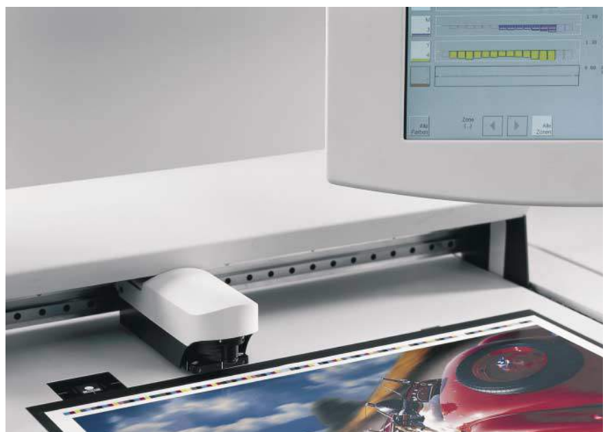
Prinect® Axis Control® is integrated in the Prinect® CP2000 Center® press control station and performs spectrophotometric measurement in the color control strip.
